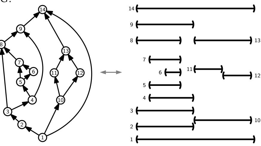
Recall that an **st-graph** is a planar digraph G with exactly one soure s and one sink t where s and t occur on the outer face of an embedding of G.
