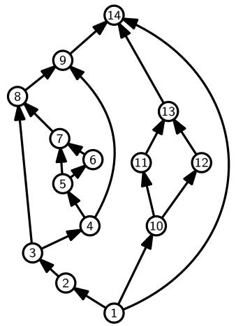
Recall that an **st-graph** is a planar digraph G with exactly one soure s and one sink t where s and t occur on the outer face of an embedding of G.
