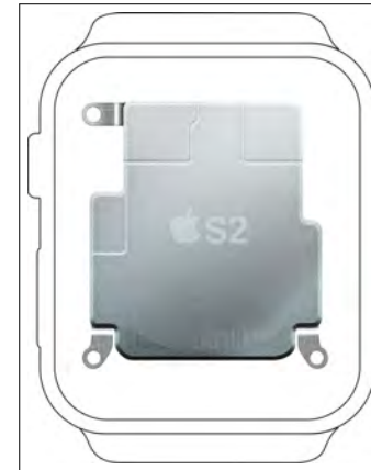
Apple S2 System-on-a-Chip (approx. 2 gigaFLOPS)
