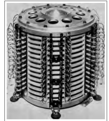
Drum memory of a Polish ZAM-41 computer
