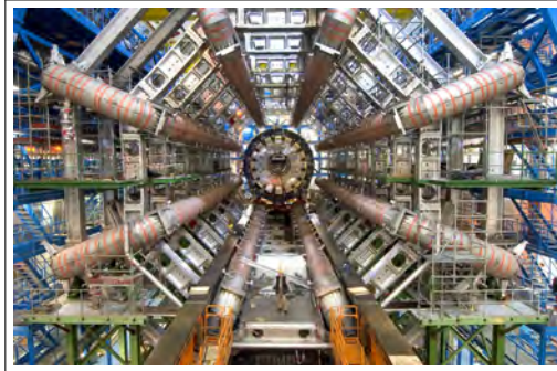
the ATLAS detector, recording data on 40 million particle-particle collisions per second at 2 MB per collision
