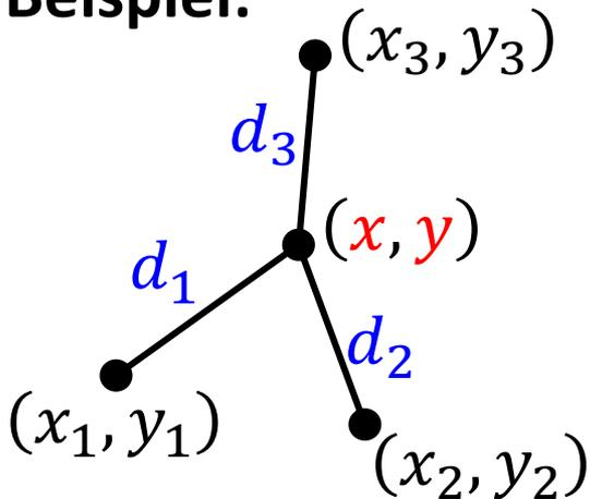
$$\begin{pmatrix} d_1 \\ d_2 \\ d_3 \end{pmatrix} = \Phi(x, y) = \begin{pmatrix} \sqrt{(x - x_1)^2 + (y - y_1)^2} \\ \sqrt{(x - x_2)^2 + (y - y_2)^2} \\ \sqrt{(x - x_3)^2 + (y - y_3)^2} \end{pmatrix}$$
