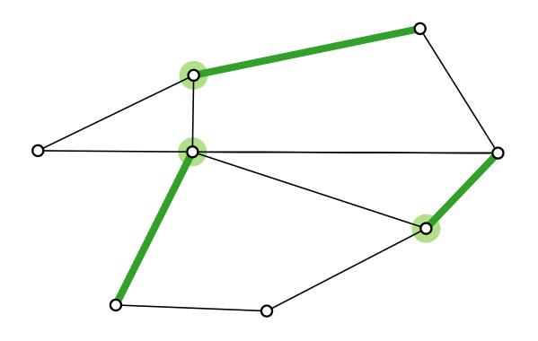
An edge set  $M \subseteq E$  of a graph G = (V, E) is a **matching** if no two edges of M are adjacent (i.e., share an end vertex).
