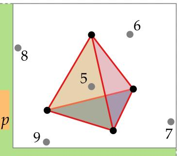
Rand3DConvexHull( $P \subset \mathbb{R}^3$ ) pick non-coplanar set  $P' = \{p_1, \dots, p_4\} \subseteq P$   $C \leftarrow CH(P')$ compute rand. perm.  $(p_5, \dots, p_n)$  of  $P \setminus P'$ initialize conflict graph G : (p, f) edge  $\Leftrightarrow$ f visible from p
