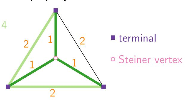
Restriction of STEINERTREE where the graph G is complete and the cost function is **metric**, i.e., for every triple u, v, w of vertices, we have  $c(u, w) \le c(u, v) + c(v, w)$ .
