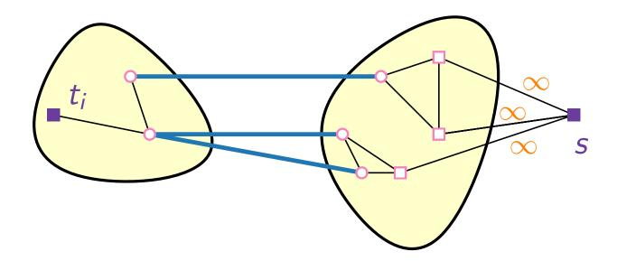
Add dummy terminal s and find a minimum-cost  $s-t_i$  cut.
