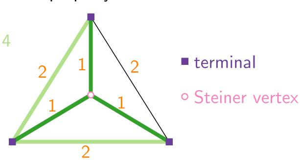
Restriction of STEINERTREE where the graph G is complete and the cost function is **metric**, i.e., for every triple u, v, w of vertices, we have  $c(u, w) \leq c(u, v) + c(v, w)$ .
